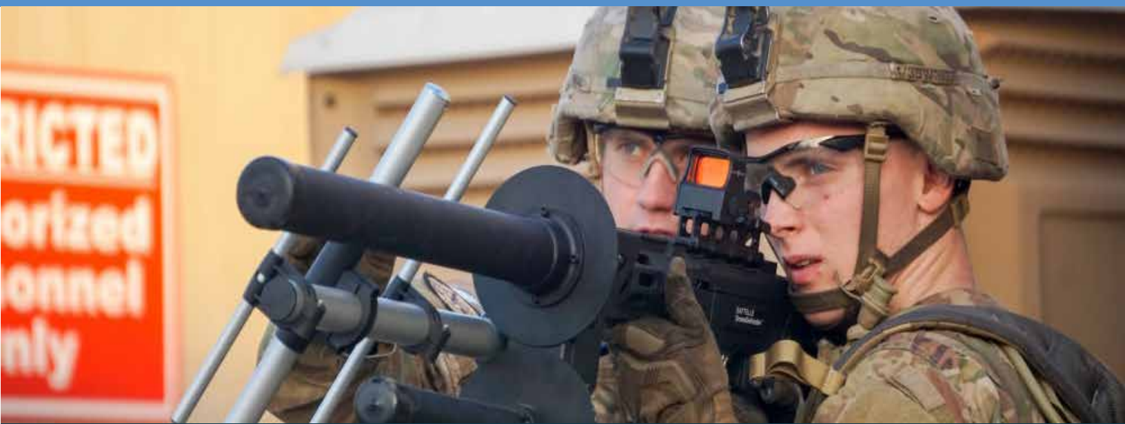
Troopers from the 3rd Cavalry Regiment operate the Drone Defender during a C-UAS drill while deployed to Iraq in 2018.
