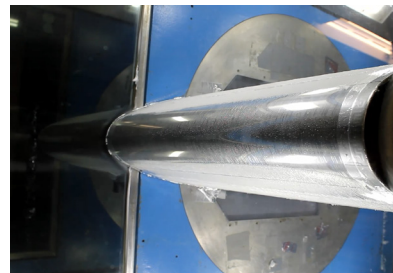
The multifunction structure is seen in Collins Aerospace’s ice wind tunnel de-icing the structure.
