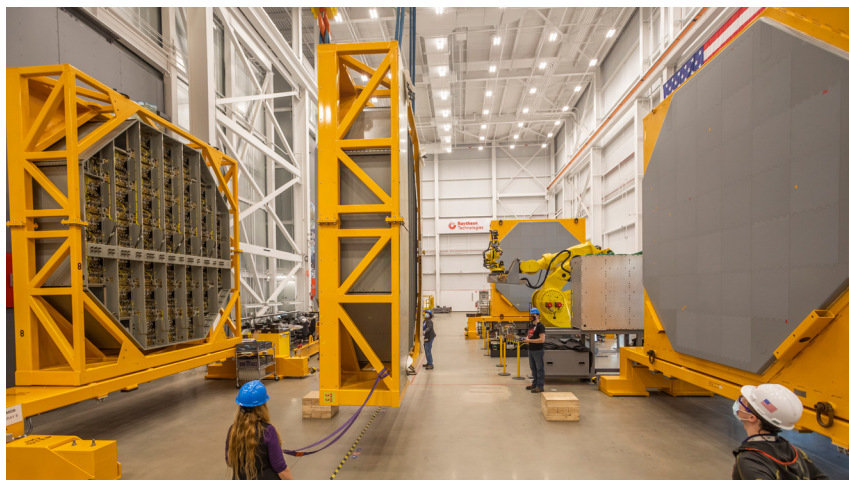
SPY-6 radar variants have between 9 and 37 radar modular assemblies, which are in and of themselves functioning radars.
