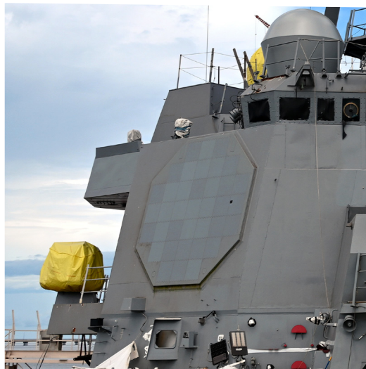
A SPY-6(V)1 radar installation was recently completed on the Navy's first Flight III destroyer, the USS Jack H. Lucas (DDG 125).
