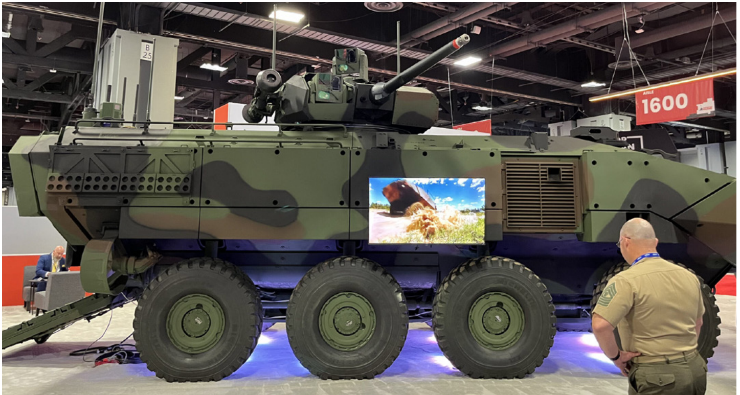
Thales' Catherine thermal image sensor is seen on the gun turret of the Amphibious Combat Vehicle, ACV-30, to provide advanced threat detection and imaging for the weapons station and crew. (Thales photo)
