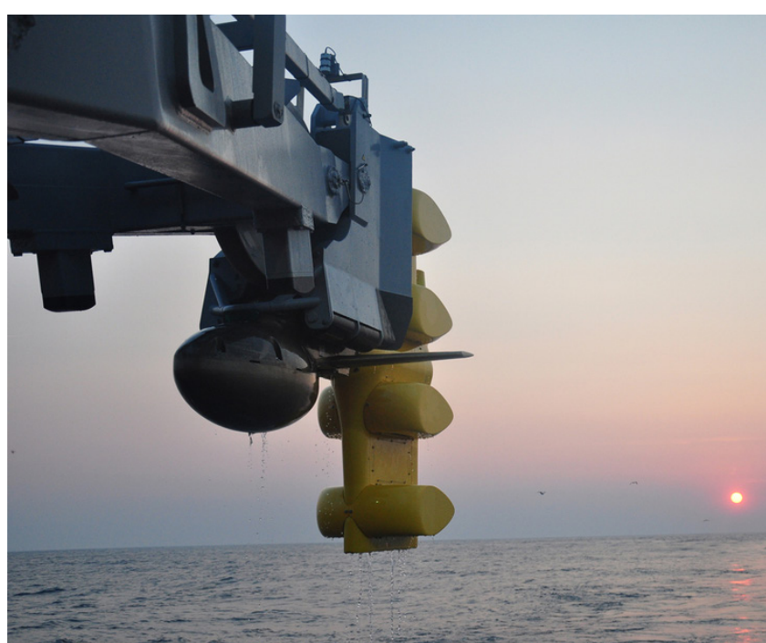
The CAPTAS-4 (Combined Active and Passive Towed Array Sonar) is built, integrated, and tested at the Thales Defense & Security, Inc. (TDSI) facility in Lemont Furnace, PA, and was selected to support the U.S. Navy's Anti-Submarine Warfare Operations. (Thales photo)
