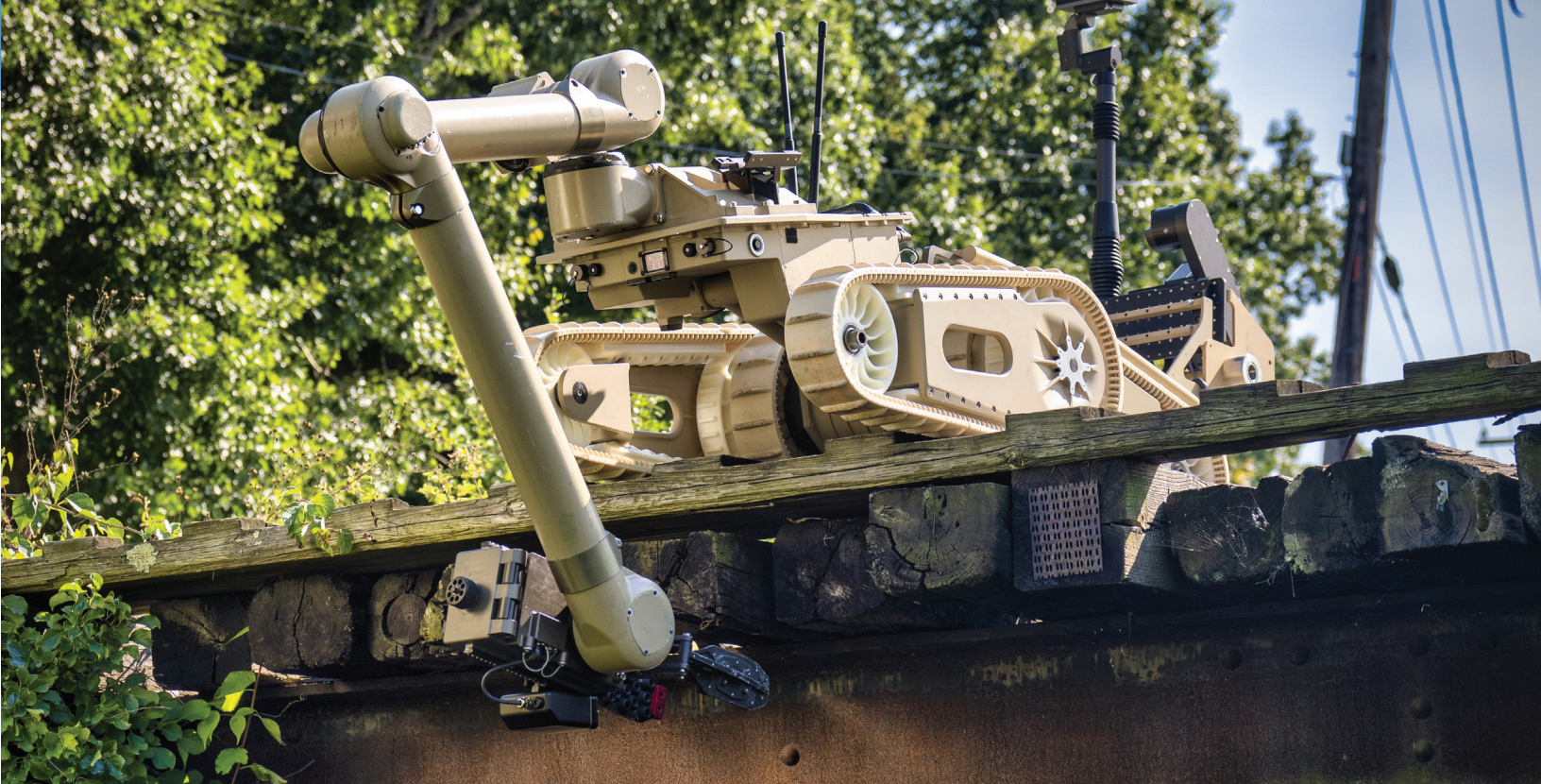
The Kobra 725 UGV can integrate and deploy a large range of accessories for EOD, CBRN/HazMat, breaching, and other applications. (Teledyne FLIR photo)
