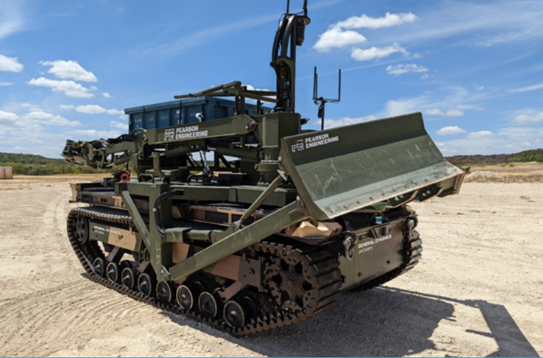
A prototype version of Pearson Engineering's RCV-Pioneer + Obstacle Clearance Mission Payload was demonstrated on the General Dynamics Land Systems TRX RCV. It included a manipulator arm capable of lifting objects up to 1,100 pounds at max range, a V-shaped dozer blade for moving obstacles, and an area which is designed to carry a variety of different loads. (Pearson Engineering photo)
