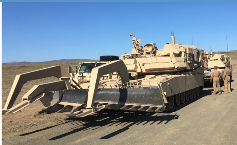
The Army is working on a tele-operation capability for the M1150 Assault Breacher Vehicle that adds a remote control system. (Army photo)
