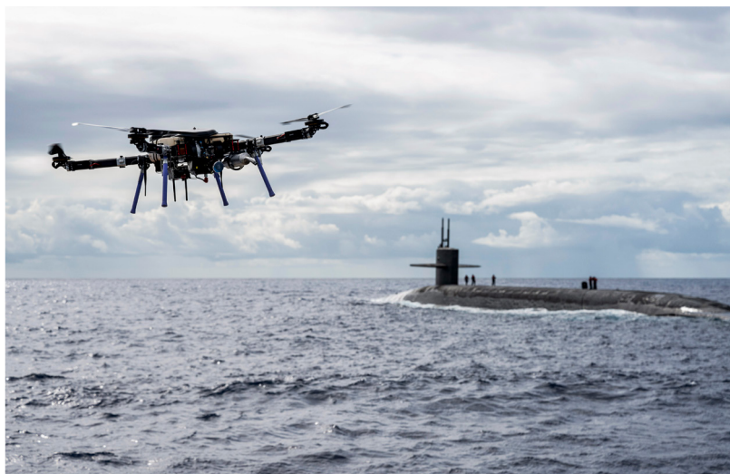
An unmanned aerial vehicle delivers a payload to the ballistic missile submarine USS Henry M. Jackson around the Hawaiian Islands, Oct. 19, 2020, during an event designed to test and evaluate the tactics, techniques and procedures of U.S. Strategic Command's expeditionary logistics and enhance the readiness of strategic forces. Photo By: Navy Petty Officer 1st Class Devin M. Langer
