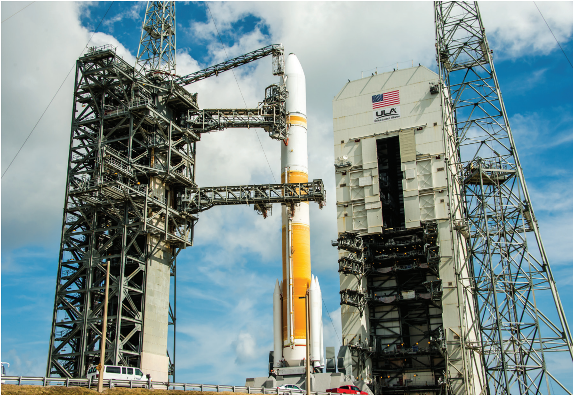
Space and Missile Systems Center's WGS-10 (Wideband Global SATCOM) encapsulated satellite mated with a Delta IV launch vehicle. The WGS constellation of SATCOM satellites operate in geostationary orbit.
