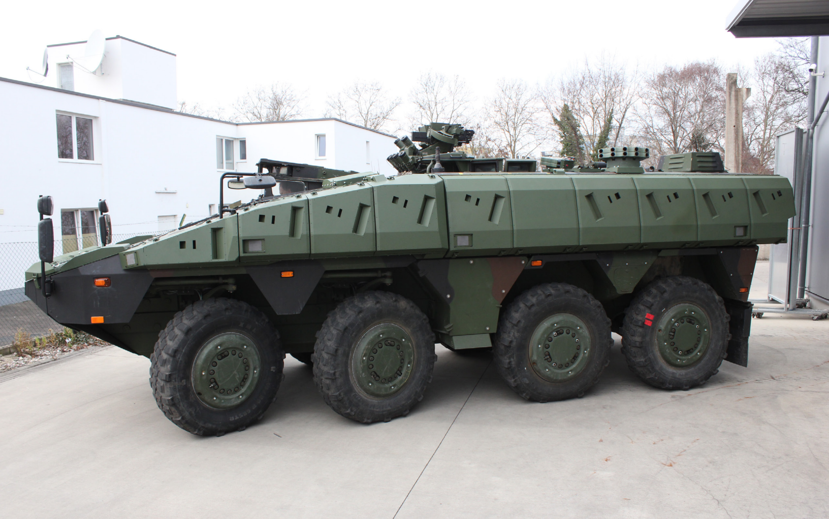
StrikeShield modular APS integration on German Boxer armored fighting vehicle.
