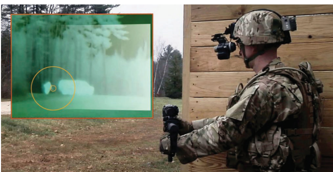
The inset image shows what the soldier can see through the wirelessly linked ENVG-III goggle and FWS-I gungight.
